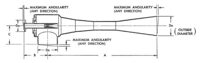
THE SAME TOLERANCES APPLY TO FLANGED CONNECTIONS AS ARE SHOWN FOR BUTT WELDED CONNECTIONS
