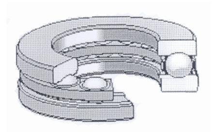
Double direction thrust ball bearings can accept axial loads acting in both directions and can thus serve to axially locate a shaft in both directions. They must not be subjected to radial load.
