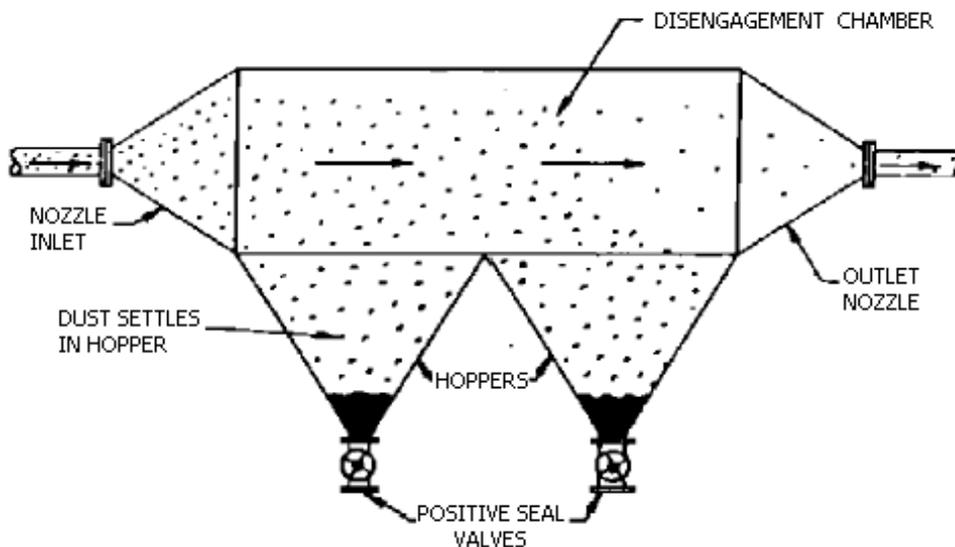
**EQUIPMENT FOR PARTICULATE REMOVAL (GRAVITY SETTLING CHAMBER)**
