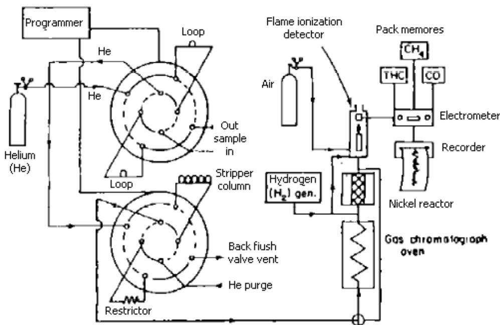
**GAS CHROMATOGRAPHIC ANALYZER FOR TOTAL HYDROCARBONS (THC), METHANE (CH<sub>4</sub>), AND CARBON MONOXIDE (CO)**
