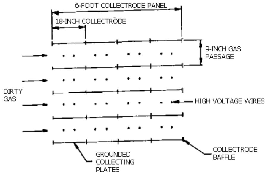
**CROSS SECTION OF FOUR-GAS-PASSAGE COLLECTRODE MODULE**
