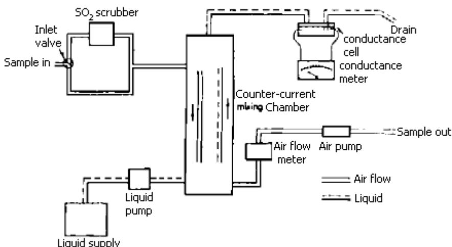
**COUNTER-CURRENT TYPE SULFUR DIOXIDE CONDUCTIMETRIC ANALYZER**
