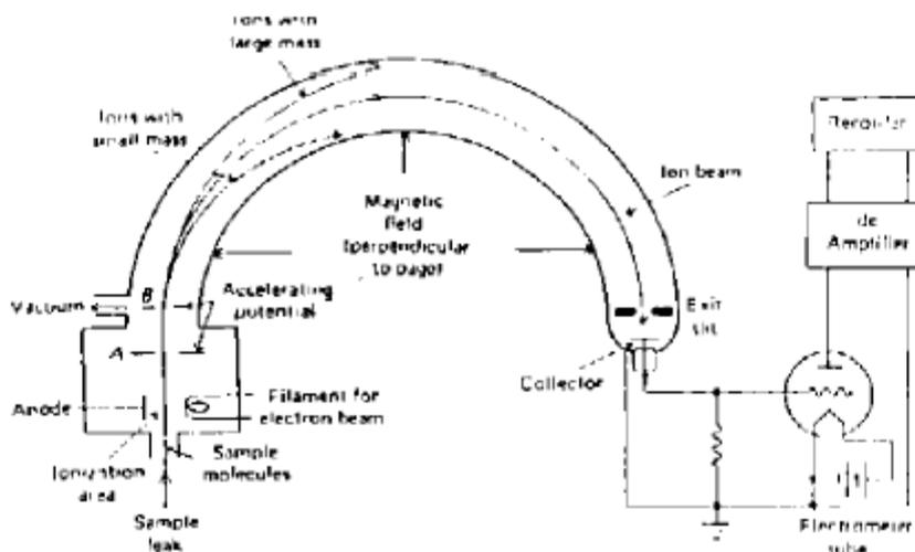
**SCHEMATIC DIAGRAM OF AN ANALYTICAL MASS SPECTROMETER.**
