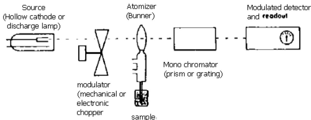
**SCHEMATIC DIAGRAM OF ATOMIC ABSORPTION SPECTROMETER**
