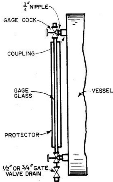
TUBULAR GAUGE GLASS CONNECTIONS TO VESSELS
