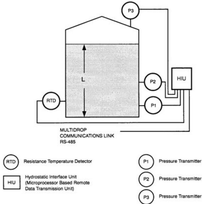
**TANK HYDROSTATIC GAGING AND INVENTORY MANAGEMENT SYSTEM**
