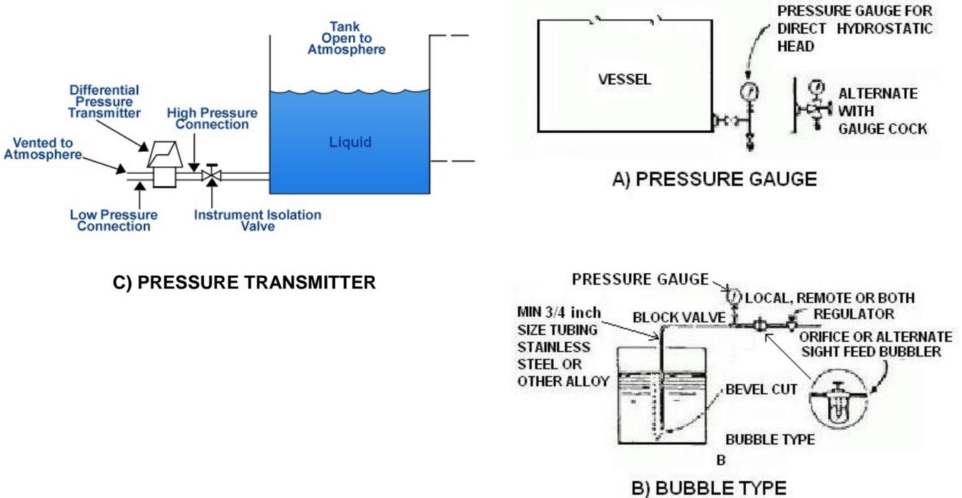
HYDROSTATIC HEAD PRESSURE GAUGE ARRANGEMENTS
