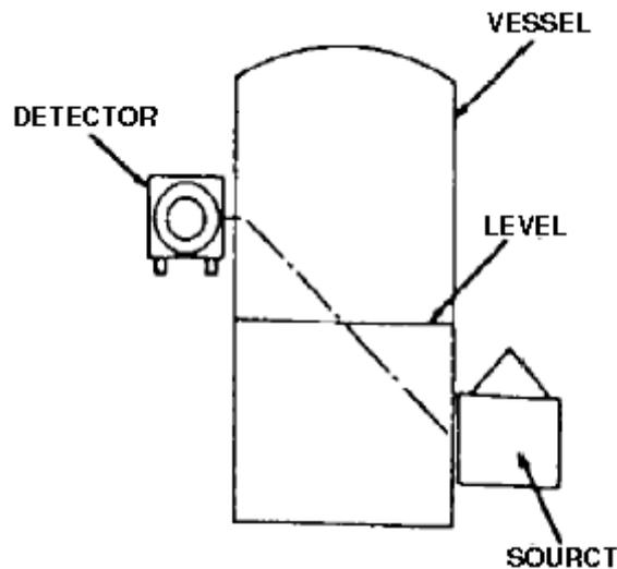
TYPICAL ARRANGEMENT OF NUCLEAR LEVEL TRANSMITTER
