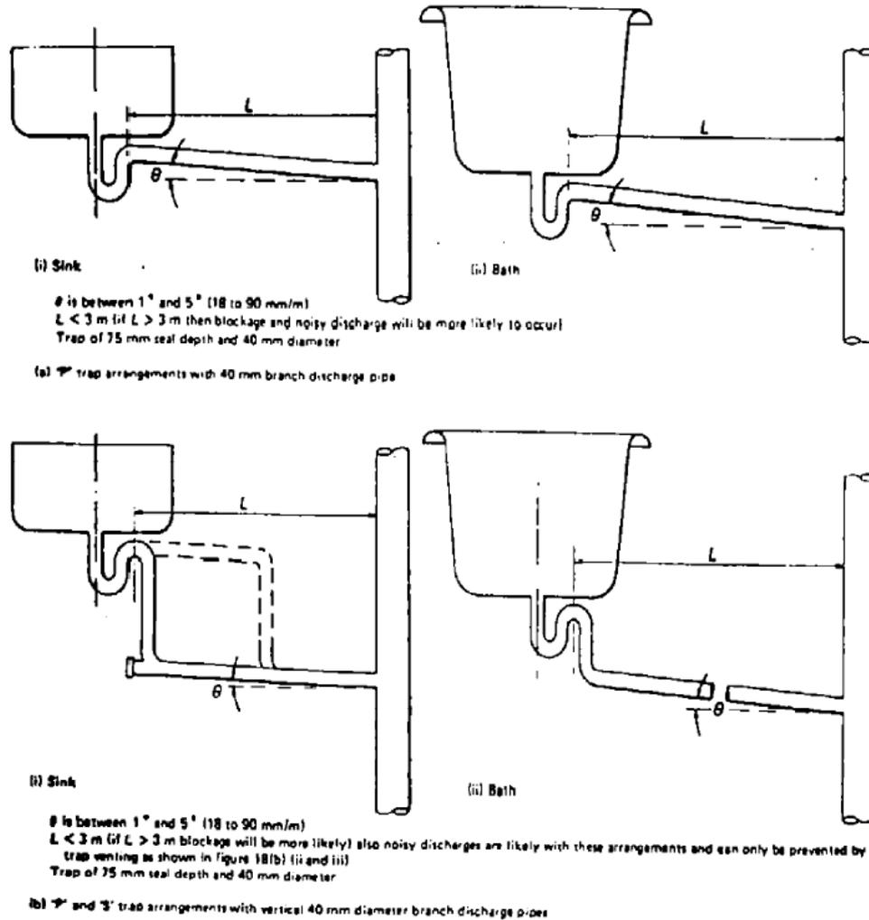
**BRANCH DISCHARGE PIPES FOR SINGLE BATHS AND SINKS**
