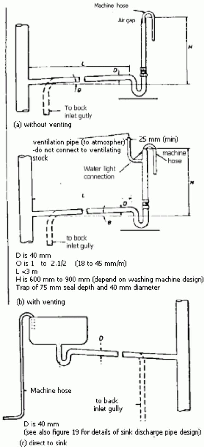
**BRANCH DISCHARGE PIPES FOR WASHING AND DISH WASHING MACHINES**
