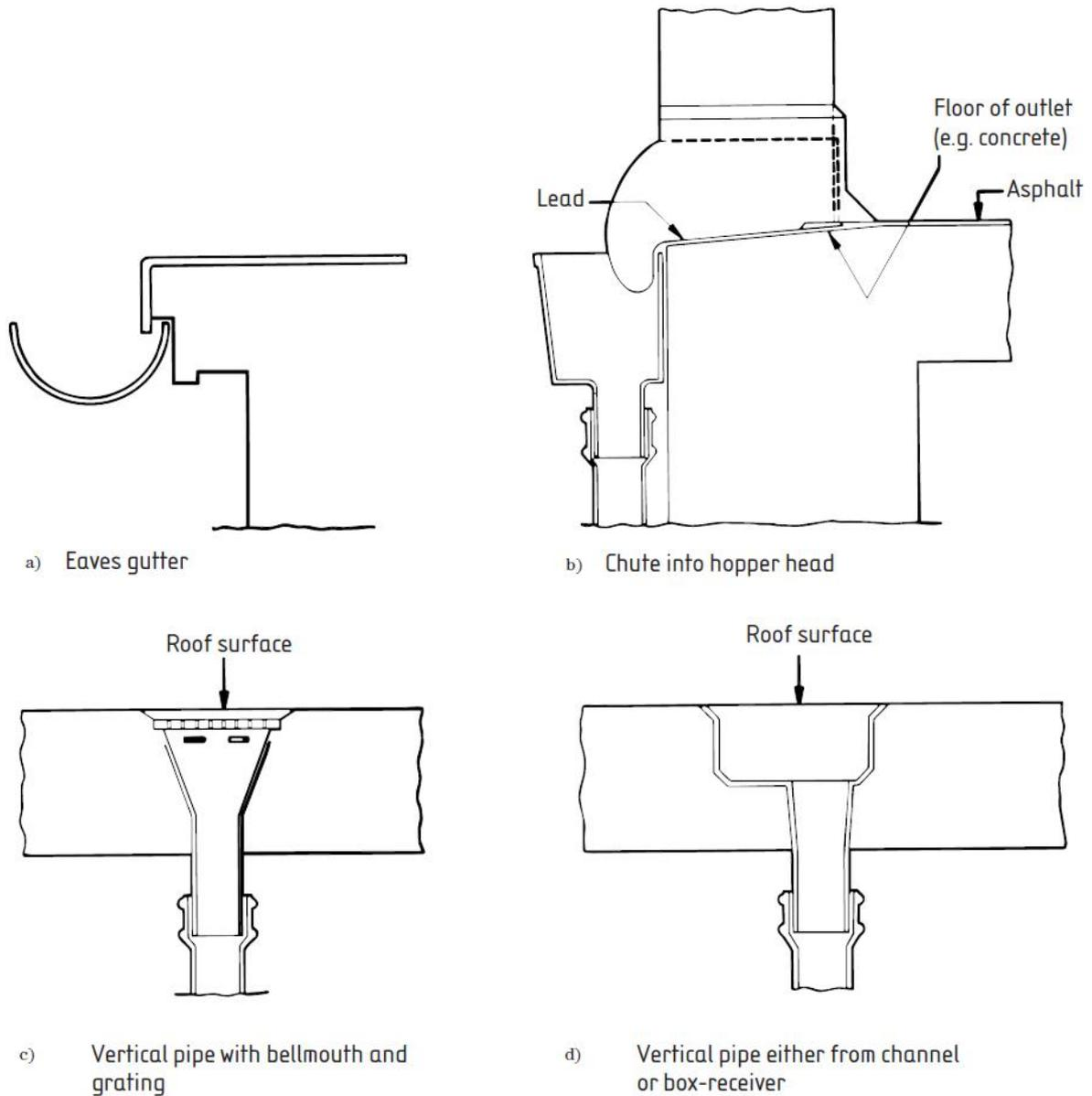
**DRAINAGE FROM FLAT ROOFS: TYPES OF OUTLET**
