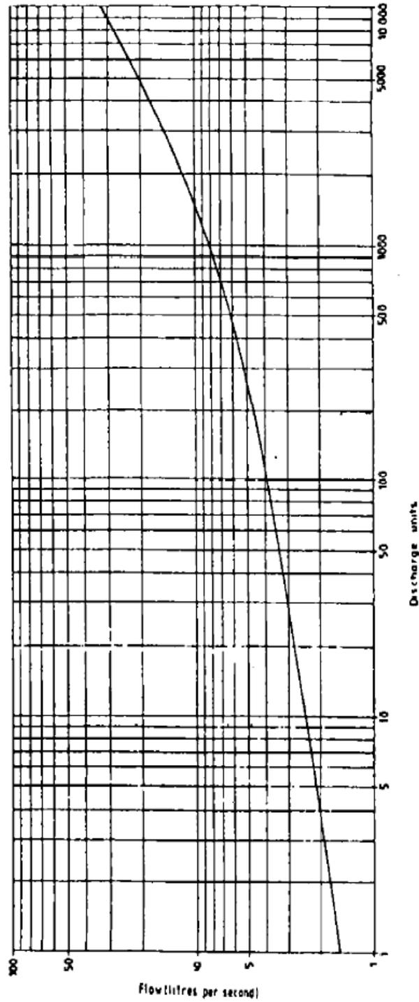
DESIGN FLOWS FOR FOUL DRAINS: CONVERSION OF DISCHARGE UNITS TO FLOW RATES
