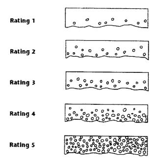
Figure 1- maximum allowable cross-section porosity
