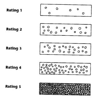
Figure 2- maximum allowable interface porosity
