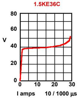
Fig 7. V/I characteristics of 36V bidirectional transzorb diode
