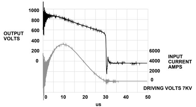
Fig 8. Let through voltage 70KA surge diverter, 900V
