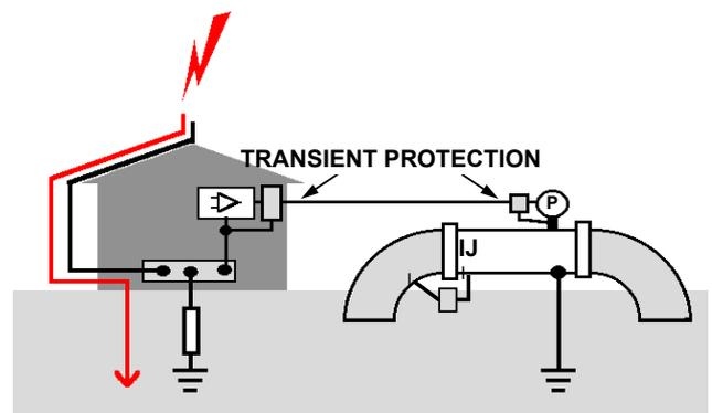
Fig 14. Instrumentation system protection
