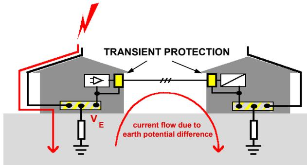
Fig 12. Signal line protection
