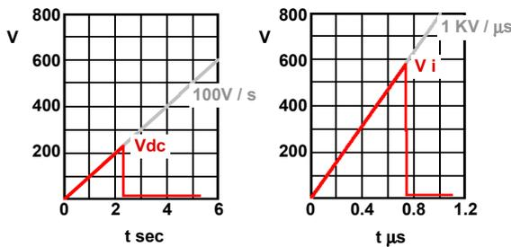
Fig 5. Gas arrester performance
