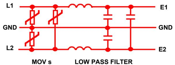
Fig 9. Mains power filter configuration
