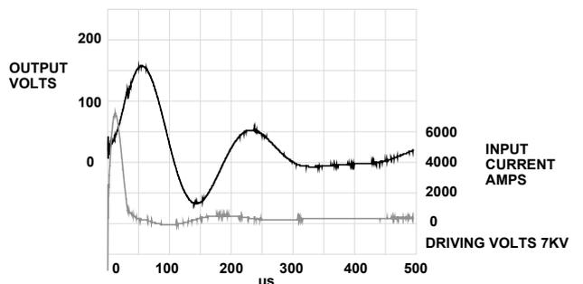
Fig 10. Mains power filter, let through 160V
