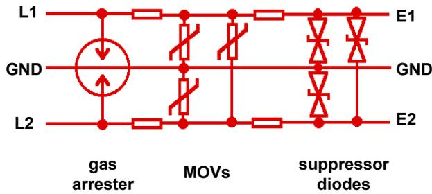
Fig 11. Multistage signal line protector
