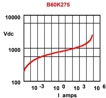
Fig 6. V/I characteristics of Siemens B60K275 MOV
