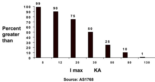
Fig 1. First stroke return current
