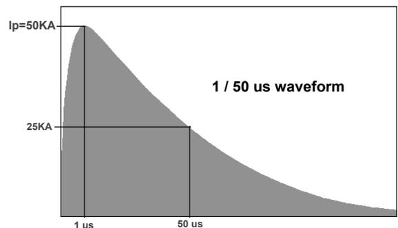
Fig 3. Lightning current waveform
