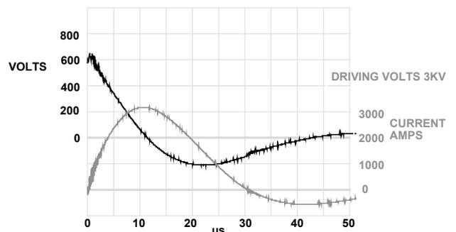
Fig 4. Voltage across 1m of 4mm<sup>2</sup> conductor
