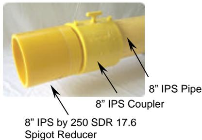
The same process is followed for the 8" imperial system, with the main difference being that the transition from the 8" to the 250mm outside diameter is achieved with a coupler and a spigot reducer rather than a dedicated electrofusion reducer as shown above.
