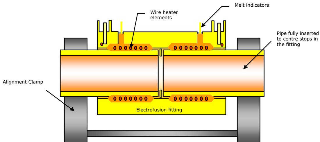
Basic procedure for electrofusion welding of solid wall polyethylene pipes
