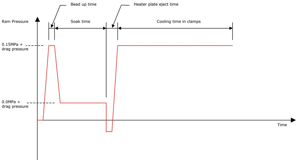
Initial bead up time reflects the requirements for the following initial bead size which is formed when the pipe end is pressed against the heater plate:
