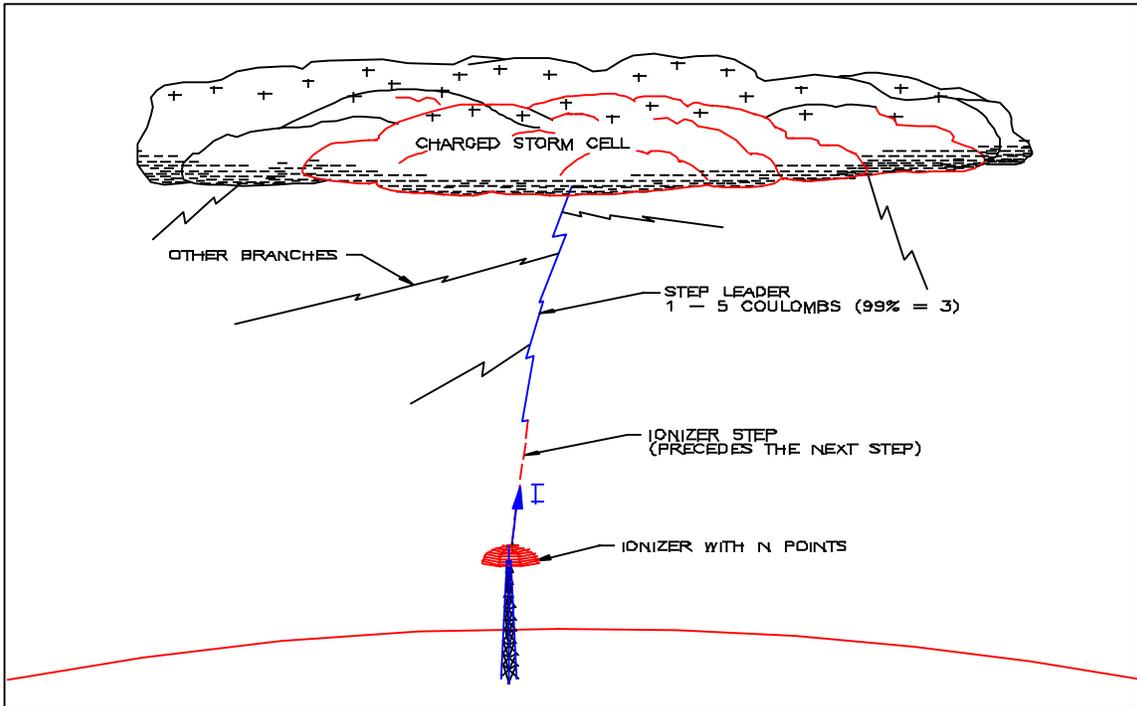
**Figure 10: Point Discharge as a Transfer Mechanism**
