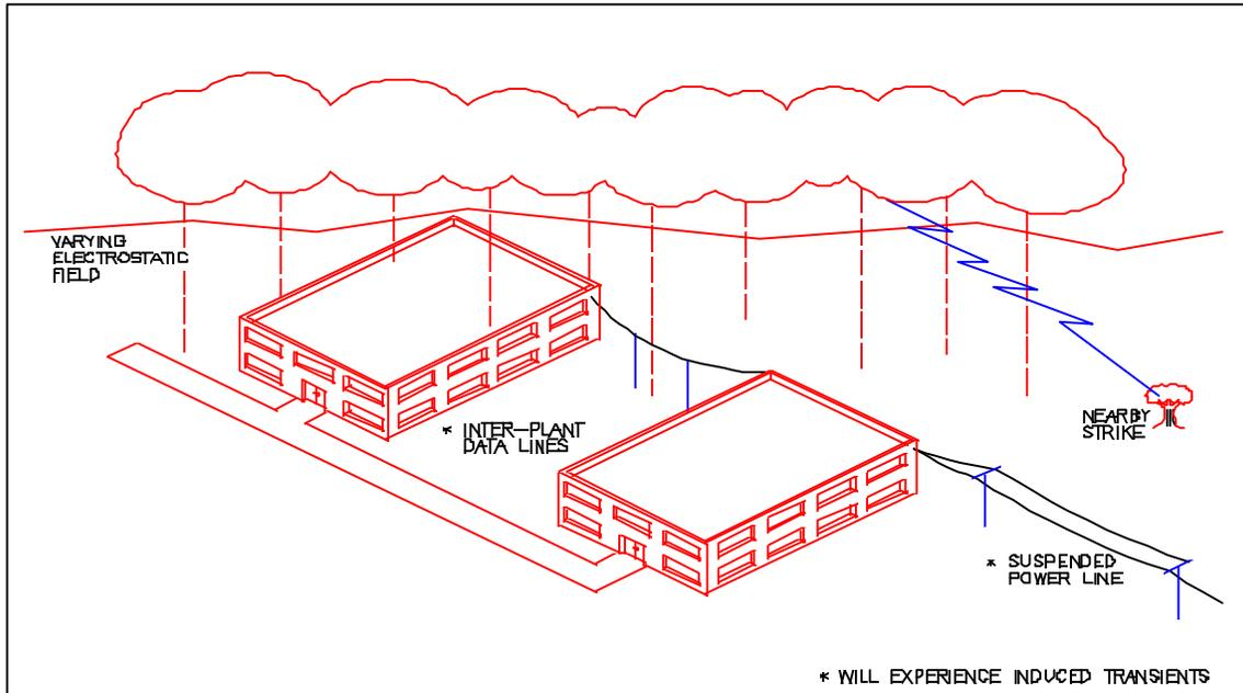
**Figure 6: Electrostatic Pulses**
