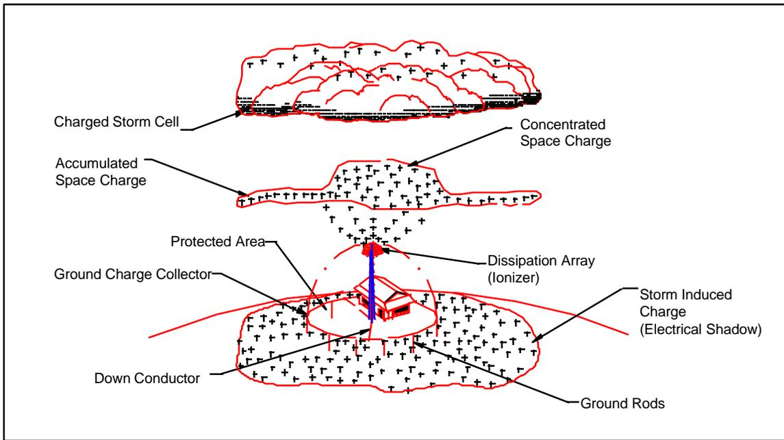
**Figure 9: LEC's Dissipation Array® Concept**
