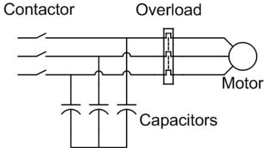
Static correction is commonly applied by using one contactor to control both the motor and the capacitors. It is better practice to use two contactors, one for the motor and one for the capacitors. Where one contactor is employed, it should be up sized for the capacitive load. The use of a second contactor eliminates the problems of resonance between the motor and the capacitors.
