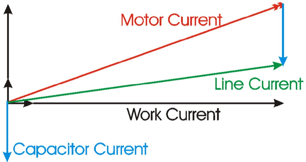
Capacitors connected at each starter and controlled by each starter is known as "*Static Power Factor Correction*" while capacitors connected at a distribution board and controlled independently from the individual starters is known as "*Bulk Correction*".
